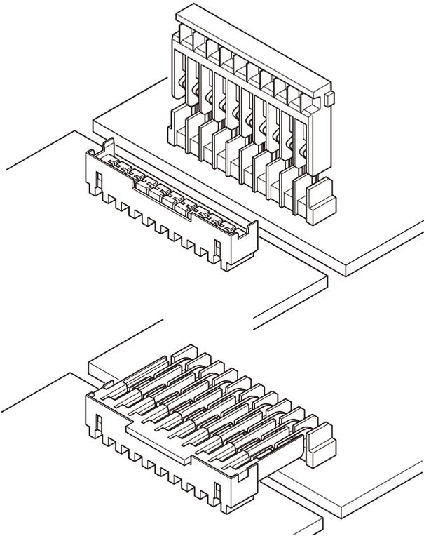
**The 2.5FJ connector is a 2.5mm pitch board-to-board connector. The connector halves can be mated after the installation of the printed circuit boards in their enclosure.**
