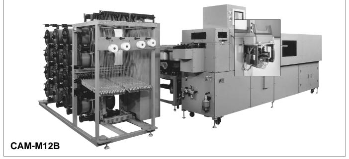
The CAM-M12B automatic machine can produce multi-harnesses. The moving chuck measures the wire lengths for each branch harness.
