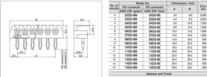
Contact: Phosphor bronze, copper-undercoated, tin-plated (reflow treatment) Housing: 2 to 11 circuits/PA 66, UL94V-0 12 to 15 circuits/Glass-filled PA 66, UL94V-0
