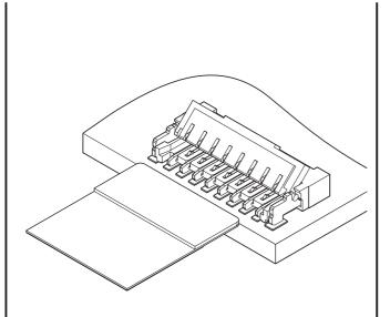
This FXVL connector is a space saving and low profile connector for FPC demanded from the market, and realizes 0.3 mm pitch connector with a mounting height of 0.9 mm and depth of 2.68 mm. In 0.3 mm pitch FPC connector, the smallest product in mounting area on the board has been provided.
