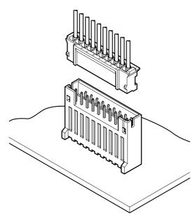
PH connector high box type, with 17 mm mounting height and with 4.5 mm thickness.
