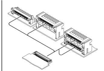
The plug consists of upper and lower parts in order to save space. This connector enables also flexible application by using either upper or lower parts individually.
