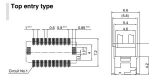
Note: 1. The above figure is the figure viewed from the connector mounting side. 2. Tolerances are non-cumulative: ±0.1mm for all centers.
