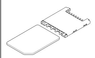
A manual insertion type connector for SIM card and Mini B-CAS card used in mobile phone
